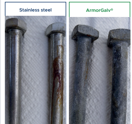
B117 Salt spray test after 1500h
